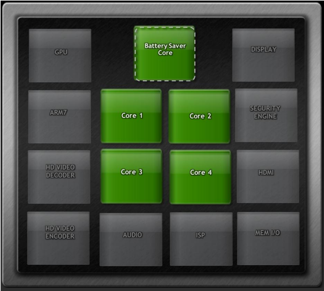
Figure 3 Low Power Battery Saver CPU on Tegra 3
